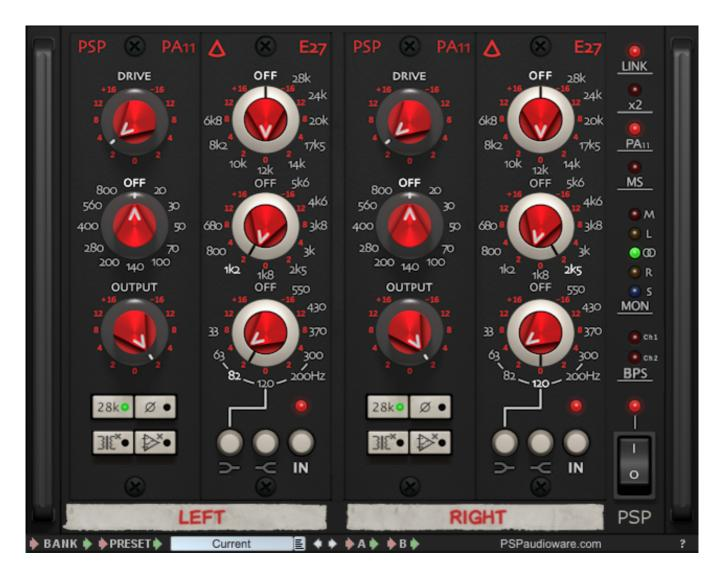
PSP E27 plugin supports three channel modes: Mono-Mono, Mono-Stereo and Stereo-Stereo. Set mono-stereo channel support in your DAW and use PSP E27 plugin with slightly different settings for Left and Right channel processing to create wide stereo field from a mono track.
