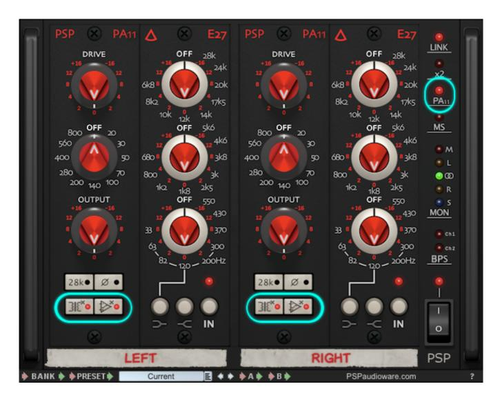
Enable TrafoX and AmpX buttons to disable the non-linear behaviour of PSP E27. This is the easiest way to get rid of distortion. This option is especially useful for mastering if there is a need to work on bands with clean linear filters. Keep in mind that the filters' characteristics and interdependency won't change.
