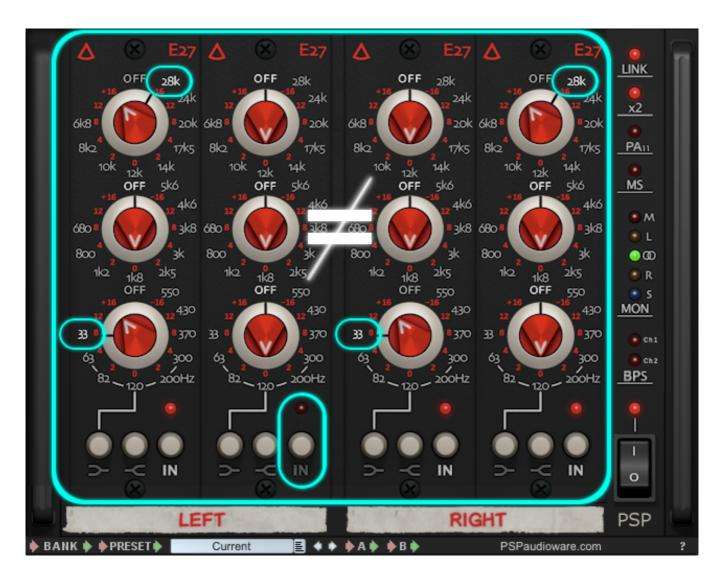
Filters within a single E27 module are interdependent and they affect on each other, due to the hardware's internal construction and the relationship between capacitors and other electronical elements. The difference between sound on the left and right setting is gentle, but audible (about 1dB).
